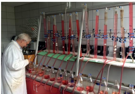
Fig. 1. Laboratory stand with model bioreactors for the tests of batch isothermal anaerobic fermentation process
