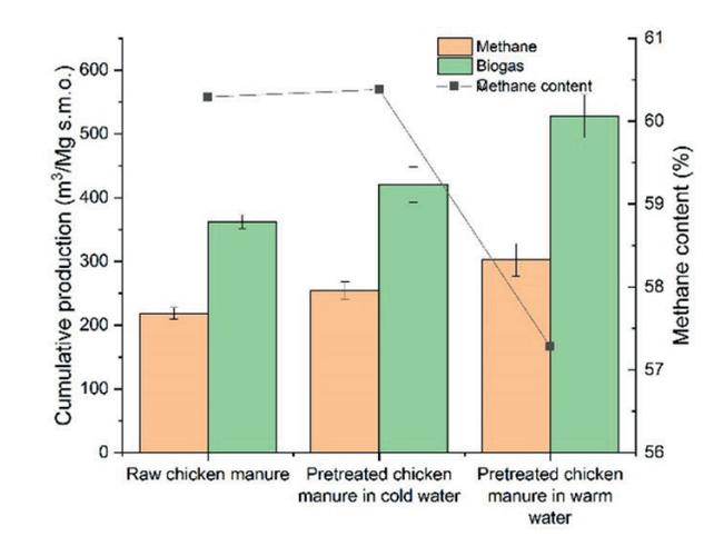
Fig. 3. Cumulative biogas and methane production for raw and pretreated chicken manure
