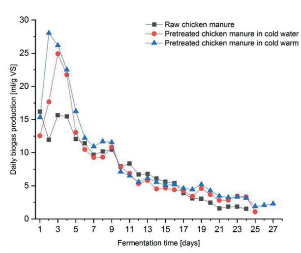
Fig. 2. Daily biogas production — raw chicken manure and pretreated
